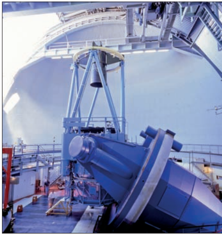
The ESO 3.6 m telescope was completely upgraded in 1999. It is equipped with HARPS, the most precise spectrograph in the world. (Image credit: HH Heyer/ESO.)
