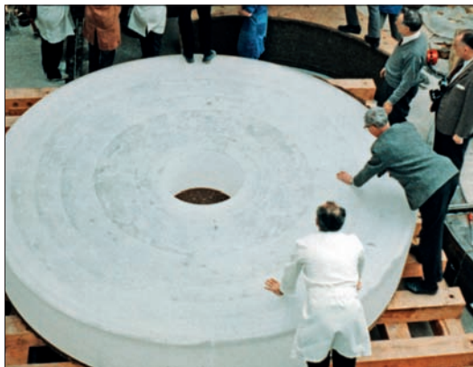
Unpacking the blank of the 3.6 m mirror at the REOSC workshops, near Paris, in 1967. (All image credits: ESO.)
