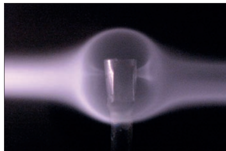
A “mini-magnetosphere” created in the laboratory. The glow is the stream of charged particles in the plasma wind tunnel. The experiment shows how a thin barrier is formed, creating a cavity in the “plasma wind” that in turn protects much of the surface of the target. (Image credit: Ruth Bamford.)
