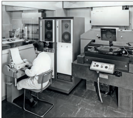
An early scanner for photographic plates, located at CERN, used for one of the first digitized surveys by the Sky Atlas Lab.
